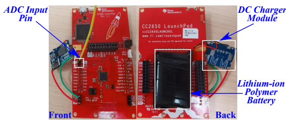
Fig. 1. The measurement device consists of a TI CC2650 Launchpad, a DC charger module, and a lithium-ion battery.
